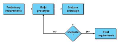
Figure 6.5 Throw-away prototyping within requirements specification
