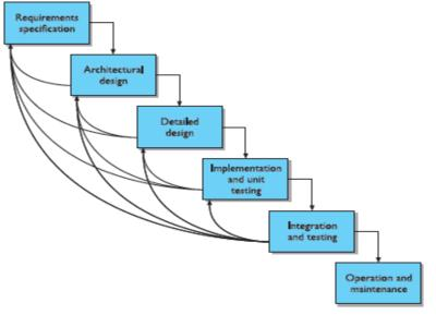
Figure 6.4 Representing iteration in the waterfall model
