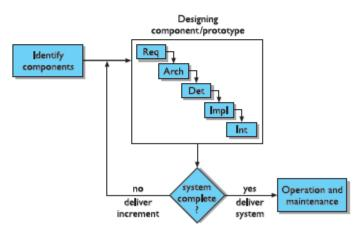
Figure 6.6 Incremental prototyping within the life cycle
