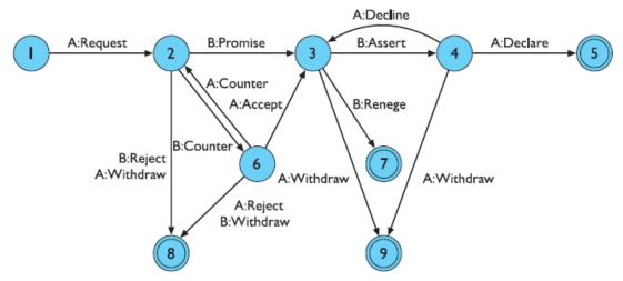
✤ The numbered circles in Figure 14.1 are 'states' of the conversation, and the labeled arcs represent the speech acts, which move the conversation from state to state. Note that the speech acts are named slightly differently in different sources (by the same author even!), but the structure of a CfA is the same. The simplest route through the diagram is through states 1–5.
